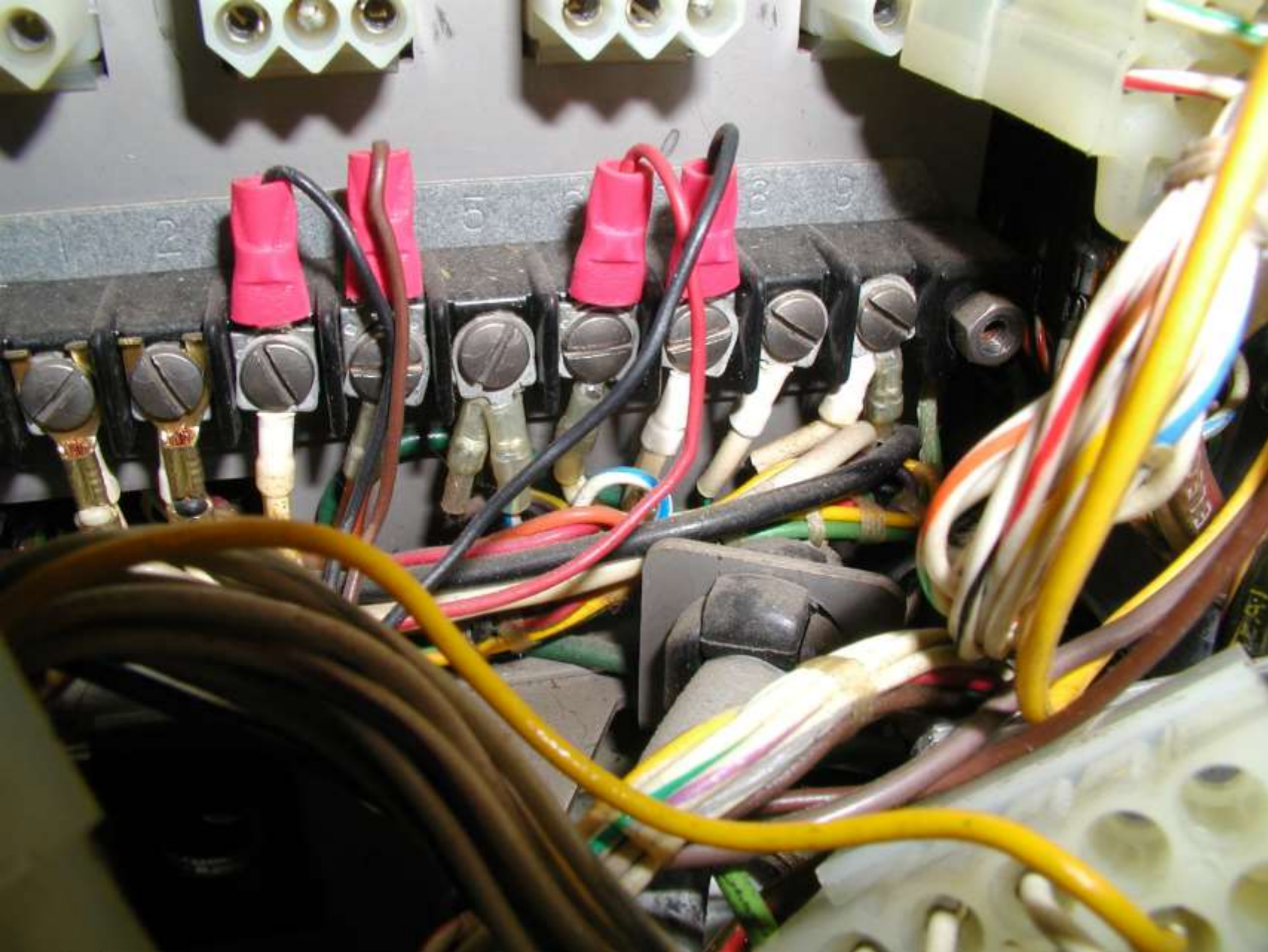
Terminal Strip is located behind the plug in connectors of the UCC-6
