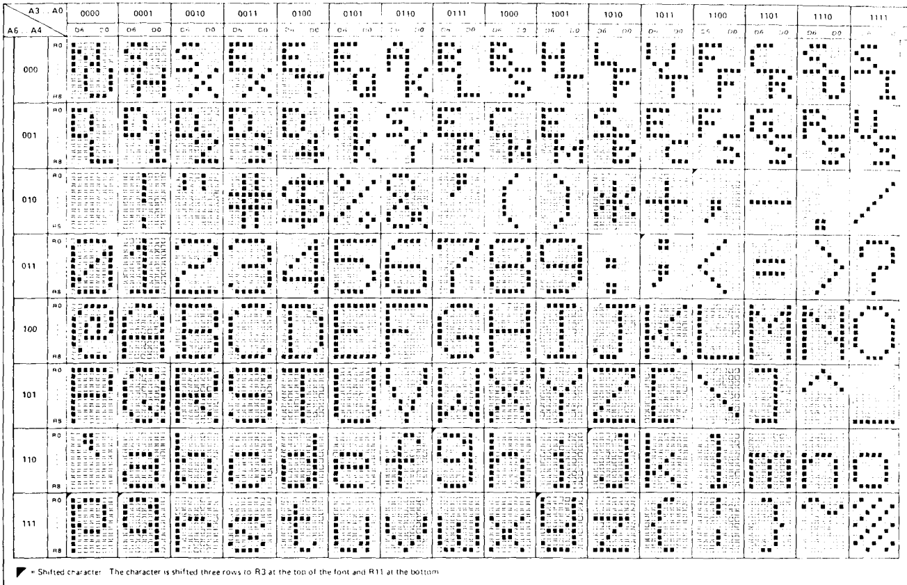
Figure 8-6. 6575 Character Generator ROM pattern.
