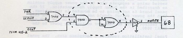
This modification should be made to your front panel board using two additional sections of the 7400 that is located directly above S-2 and S-3. This will keep your unit from writing into memory during an output.
