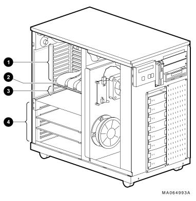
Figure 2-5 System Module Locations
