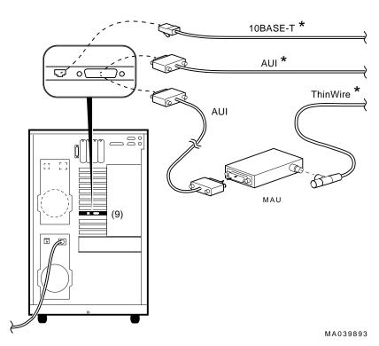
Figure 1–10 Ethernet Network Connections
