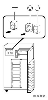
Extended Power-Down (AC Power) If an extended power-down is required, first turn off DC power as described in the previous section. Next, turn off AC power and remove the system power plugs from the power outlets as shown in ① and ② in Figure 1–9:
