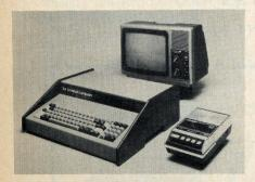
Processor Technology's Sol System was one of the first of the all-in-one computers that don't require connection to a separate (and usually costly) terminal. A single typewriter-sized cabinet contains the CPU and memory, a video interface (with upper/lower case, reverse video and some graphics
